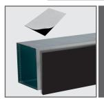
Peel back release paper & fix the sheet in line with duct edge. Press firmly to energize adhesive.
